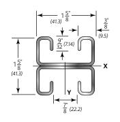
1<sup>5</sup>/<sub>8</sub>" x 1<sup>5</sup>/<sub>8</sub>" (41.3mm x 41.3mm)
